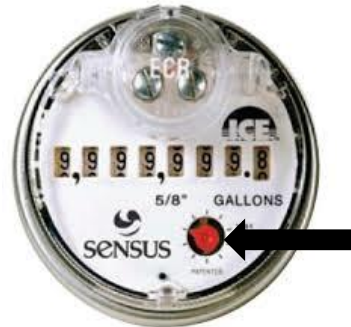
Leak Indicator: Red dial with a arrow point on it
