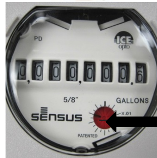
Leak Indicator: Red dial with a black line
