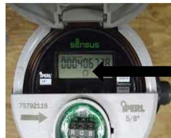
Leak Indicator: Circle in center under the numbers (Water movement is noted by a positive symbol (+). If a negative symbol (-) is present, water is moving backwards through the meter, known as "backflow".)
